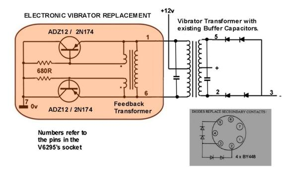
The circuit results in the vibrator transformer itself and its magnetic properties determining the frequency of oscillation. Typically, run in this mode, the vibrator transformer, designed for 120Hz operation, runs along in the region of 50Hz to 70Hz:
