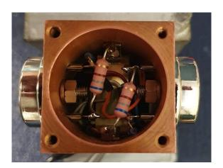
Due to the fact, with this circuit configuration, the Transistor collectors are grounded, that avoids the need for any insulating washers and gives a very good thermal and electrical bond between the transistor's collectors and the Copper housing. It is hard to see in the photo, but the transistor B & E wires are insulated with clear heat shrink sleeving.
