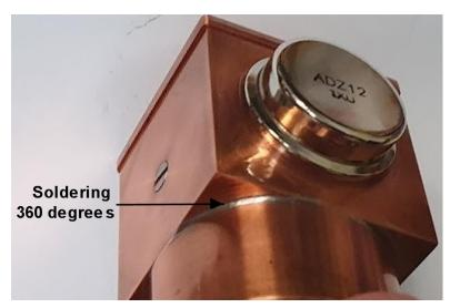
I wanted to keep the Copper finish because of its somewhat Steam-Punk look so I lacquered the body with clear Dupli-Color spray (except where the transistors mounted) This paint product is extremely adherent to shiny metals. But where the vibrator plugs in there is a metal earthing clip. For that I Silver plated it with a rubbing solution typically used for restoring vintage silver plated Tea Pots.
