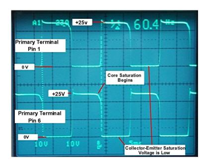
Also in this instance the "slow" Germanium power parts have a significant advantage, apart from their low Collector-Emitter saturation voltage drops of below 200mV, they have a long storage time in the order of 20uS.
