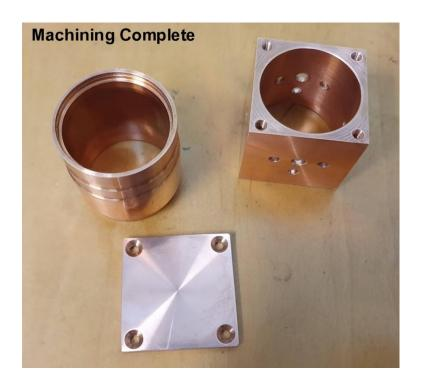
The screw threads are 1/8 BSW, this is a good size for soft metals such as aluminium or copper. It has a thread pitch similar to a 4-40 UNC, but is 1/8" (3.175mm) diameter, vs the 2.75mm diameter of the 4-40 screw.
