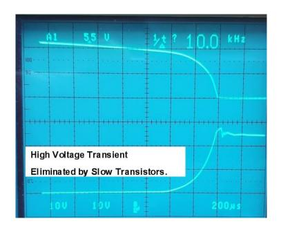
Hi performance "fast" Germanium power parts are available, a good example being the 2N1908 which have low storage times in the vicinity of only 1.5uS almost rivalling some Silicon parts. However for this application I would not recommend these. It is much better to use the slower parts with storage times in the 20uS region. Mostly these suitable transistors are the ADZ12, 2N174, ASZ16, ASZ17 and NKT404, which were devices intended for Audio and low speed switching applications.
