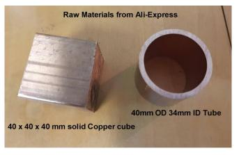
I realized I would not be able to machine the whole object as it was 76 mm long sans the 3mm thick lid. So I decided to make it in two halves and machine a 6mm long overlap to fit them together and then solder them.
