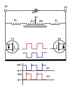
Figure 1, above is a recording of the situation seen using modern fast parts, such as Silicon power Transistors or Mosfets and a close examination of the switching with the delay time-base. These modern parts switch synchronously on and off in very short time frames in well under 1uS. As a result the high voltage from the
