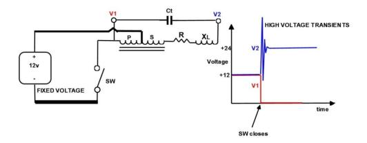
With typical vibrator transformers, when the primary halves are switched rapidly, the first positive half cycle of the leakage inductance related oscillations begins about 8uS after the Transistors (or Mosfets) change their switching state and appear on the primary terminal and the device which has just previously rapidly switched off, effectively uncoupling itself from that primary terminal. The main initial transient is over by about 16uS.
