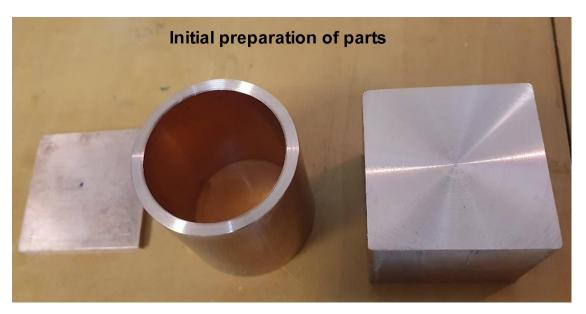
To get started I faced the end edges of the cylinder and the copper cube.
